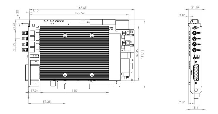
Dimensions are in millimeters.
