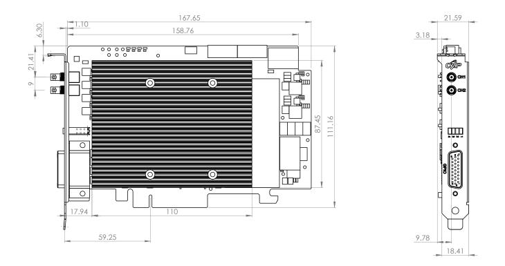
Dimensions are in millimeters.
