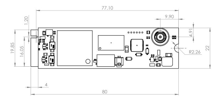
Dimensions are in millimeters.
